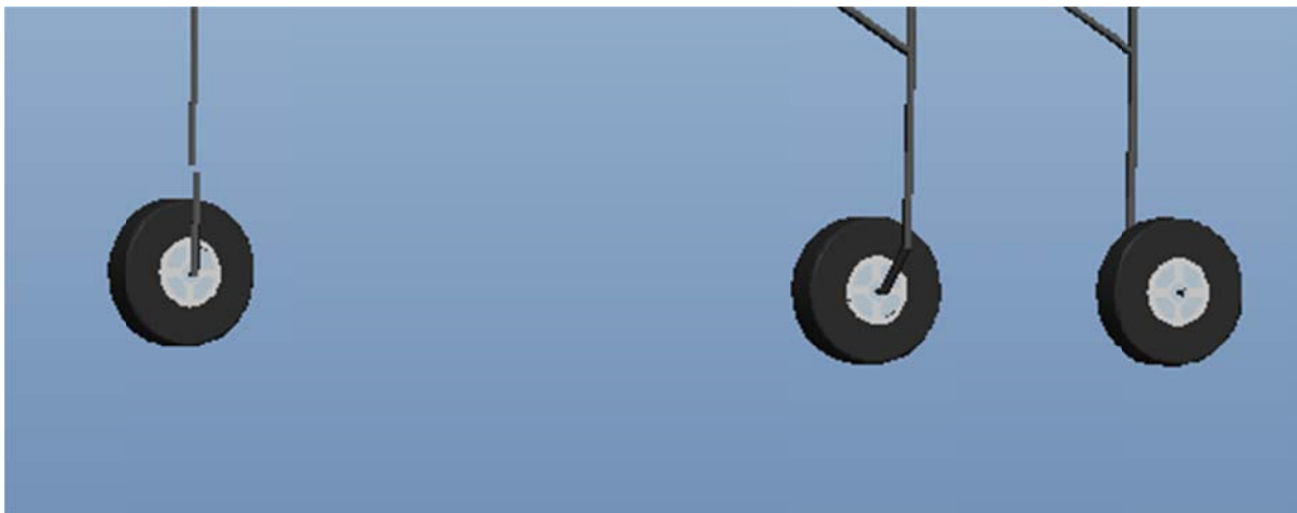
Figure 28 shows a 3-d model of our landing gear, which shows a toe of zero and a camber of zero to minimize taxi roll resistance at take-off.
